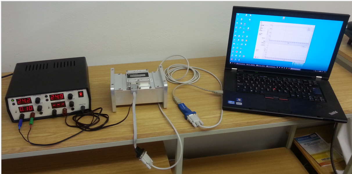
Fig. 17. Illustration of BPM – PC connection.
