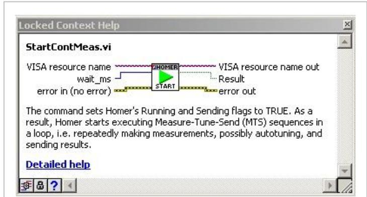
Fig. 3. Example of a LabVIEW virtual instrument block.
