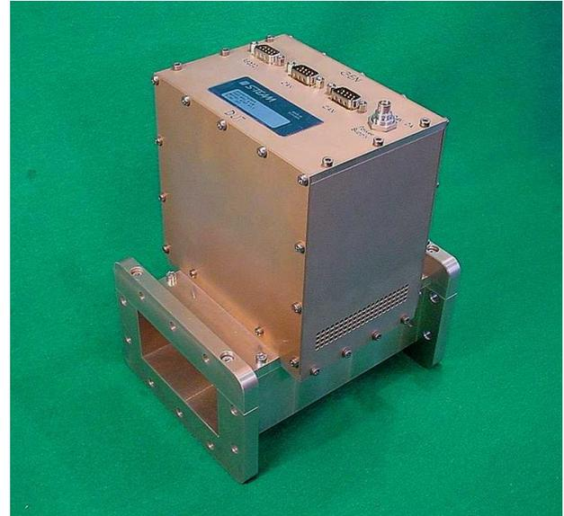
Fig. 1. HOMER STH Analyzer (2.45 GHz, WR-340 waveguide).
