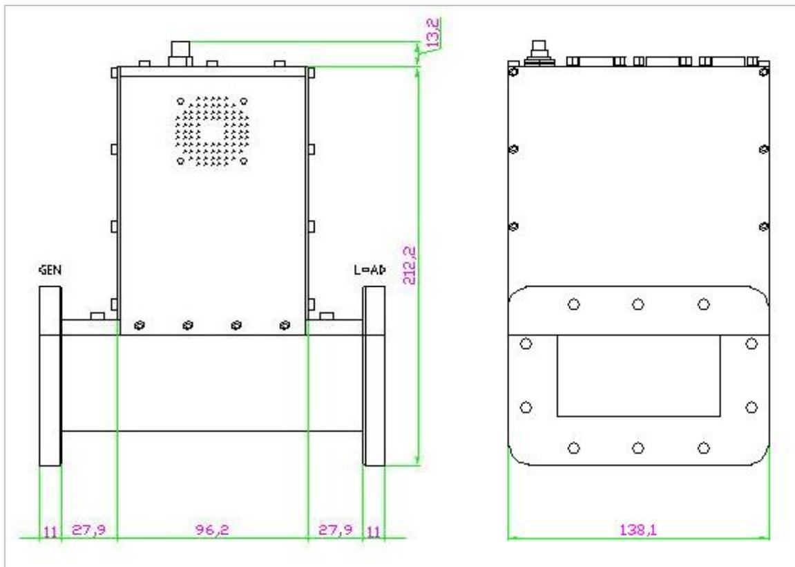
Fig. 4. Basic HOMER Analyzer dimensions. All dimensions are in millimeters.
